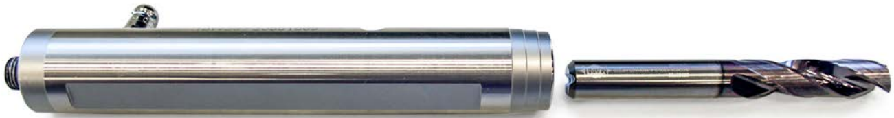
The custom hydraulic chuck and a drilling tool with a cylindrical shank; the connections located at the back to improve accessibility can also be seen.
