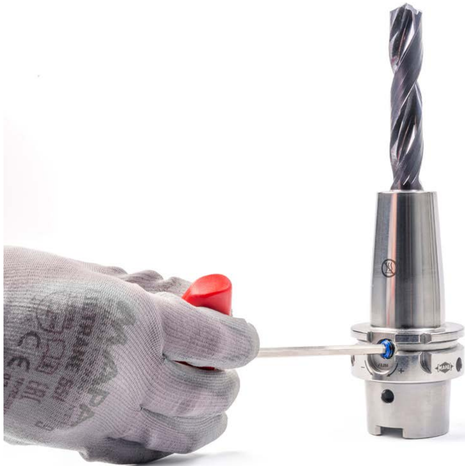
It only takes about two minutes to change a tool with a hydraulic chuck.
