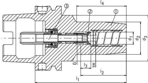
① Hydraulic chucks, HSK, MQL, body material | BDY
