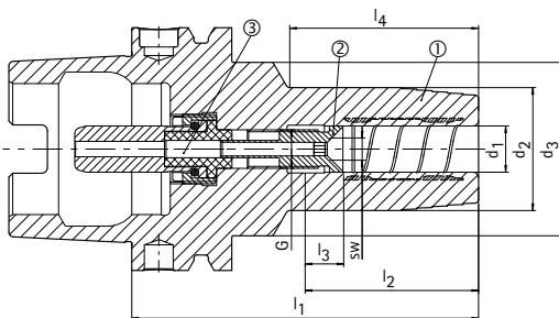
① Hydraulic chucks, HSK, MQL, body material | BDY
