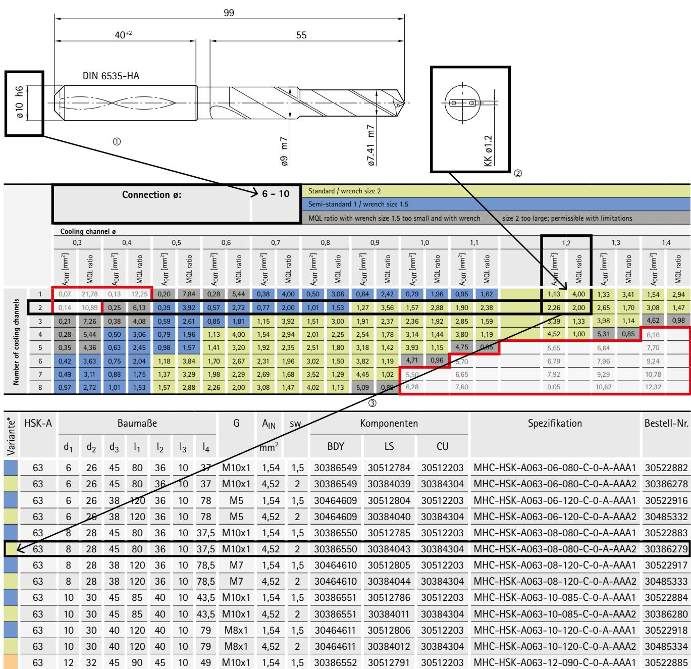
Calculation of the MQL ratio taking into account the inlet cross-section  $A_{IN}$  Semi-standard 1 variant.
