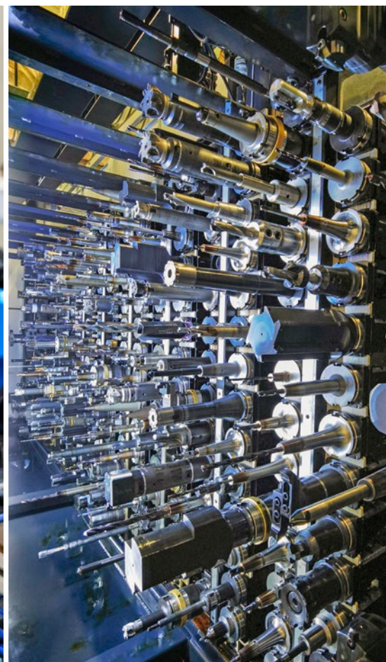
The tool magazine of the milling machining centre provides space for around 300 tools.
