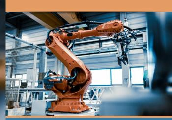
Round steel bars with a diameter of 30 to 100 mm and a length of 300 to 2,000 mm are machined on the system from Mössner. A robot is in charge of loading and unloading the system. © GABO STAHL
