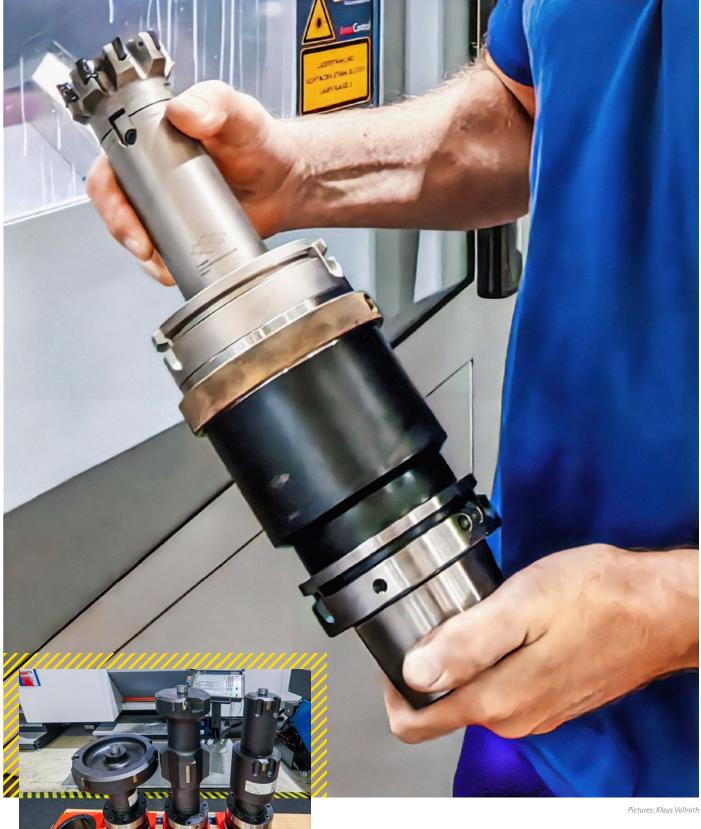
The NeoMill-4-Corner with an extension is used for roughing all larger bores. MAPAL was able to reduce the operating time from 34 to 16 minutes thanks to an optimised milling strategy.
