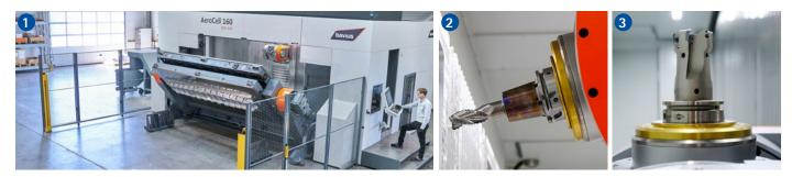
1 The bavius horizontal machining centre AeroCell 160 for the high-speed machining of aluminium structural parts up to 1600 x 4000 mm. © bavius
