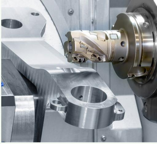
MAPAL deploys the NeoMill-Titan-2-Shell for the trochoidal milling of a torsion link.
