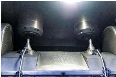
Neapco\_3: The raceways of the forged axle spindles are hard milled on the twin-spindle machining centre EMAG VSC 250 Twin.
