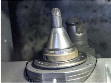
Neapco\_8: The ball nose milling cutter with four soldered-in PcBN blades removes between 0.2 and 0.4 mm of material during machining.
