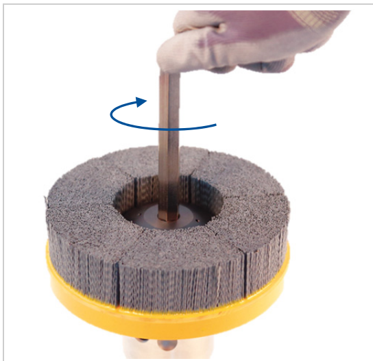
Figure 4: Tighten the clamping screw finger-tight up to the stop
