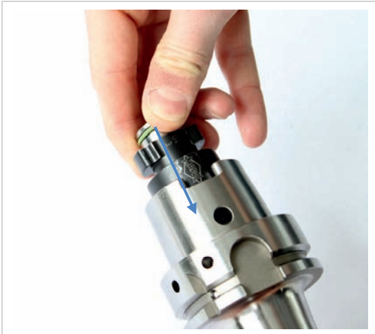
Figure 7: Testing KS clamping cartridge with tool
