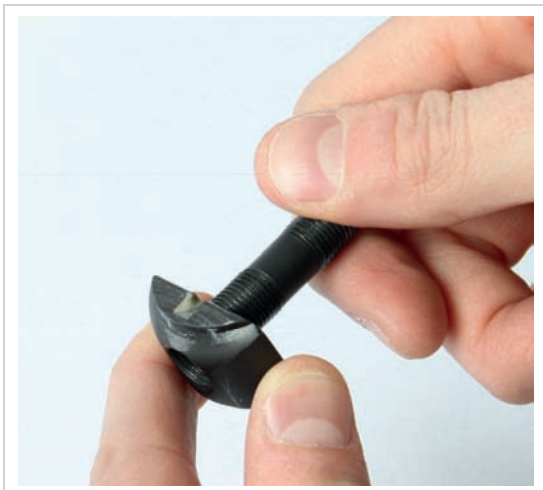
Figure 4: Screwing the threaded spindle into the smaller clamping jaw
