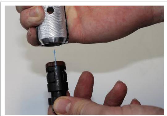
Figure 5: Inserting the KS clamping cartridge into the KS assembly pliers.
