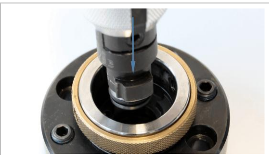
Figure 6: Inserting the KS clamping cartridge
