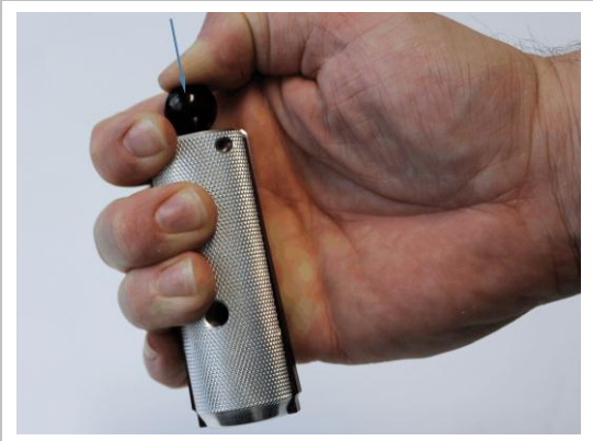
Figure 4: Open the KS assembly pliers
