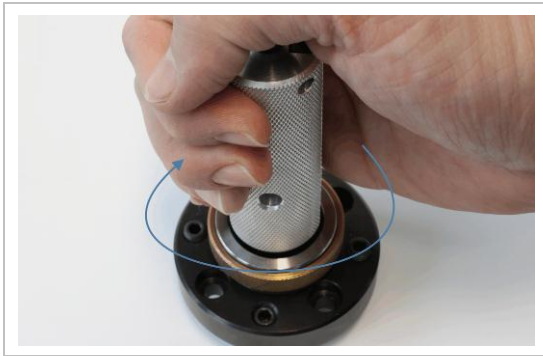
Figure 7: Arresting the KS clamping cartridge
