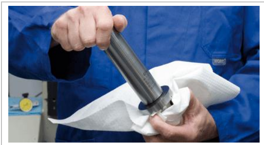
Figure 9: Cleaning the tool shank
