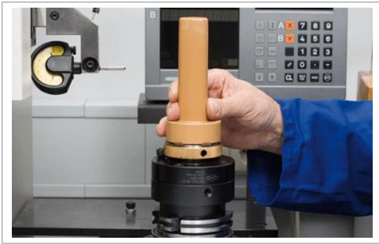
Figure 8: Cleaning the HSK interface
