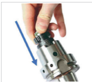
Fig. 27: Testing KS clamping cartridge
