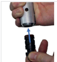
Fig. 7: Inserting the KS clamping cartridge into the KS assembly pliers.
