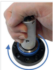
Fig. 9: Arresting the KS clamping cartridge
