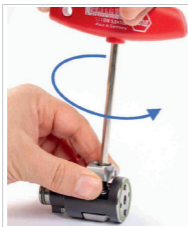
Fig. 26: Screw in the threaded spindle
