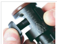
Fig. 18: Fitting the threaded spindle
