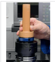
Fig. 10: Cleaning the HSK interface
