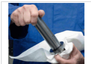
Fig. 11: Cleaning the tool shank
