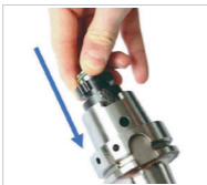
Fig. 20: Testing KS clamping cartridge
