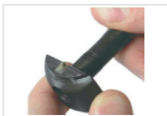
Fig. 17: Screwing the threaded spindle
