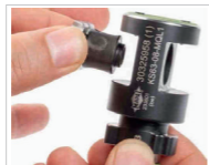
Fig. 24: Fitting the clamping jaw (3)
