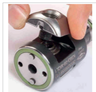
Fig. 25: Fitting the threaded spindle
