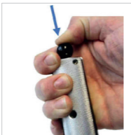
Fig. 6: Open the KS assembly pliers
