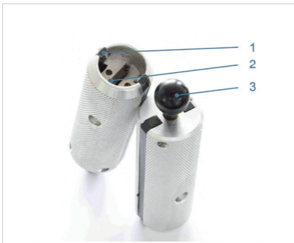
Fig. 5: Individual components of the KS assembly pliers for MQL design
