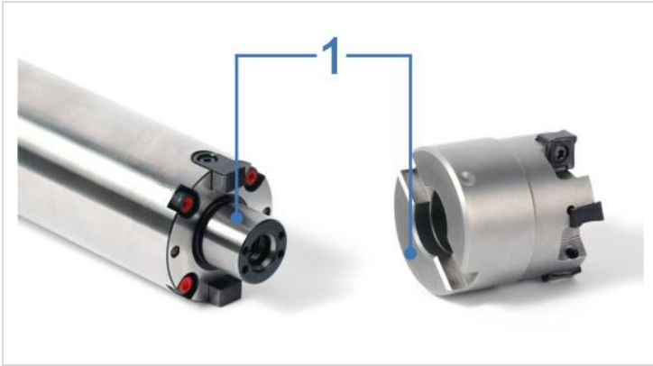
Fig. 2: Cleaning milling cutter arbor and tool
